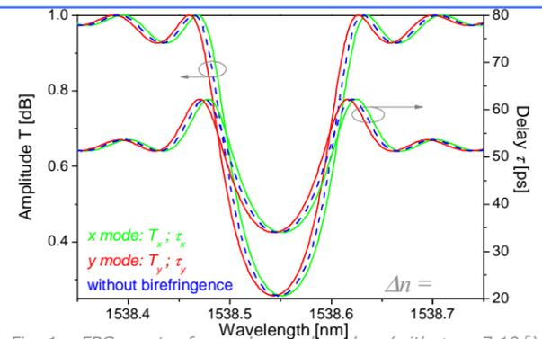
Fig. 1 – FBG spectra for mode x and mode y (with  $\Delta n = 7 \cdot 10^{-5}$ ) and for FBG without birefringence
