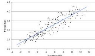
Figure 6: correlation between P<sub>EVAP</sub> and T<sub>OUTDOOR</sub> for one year measurements
