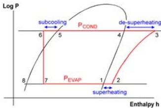
Figure 1: refrigerant cycle
