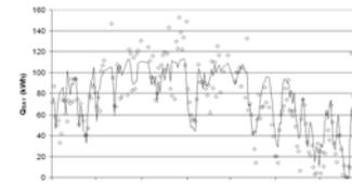
Figure 8: Q<sub>DAY</sub> measurements (◇) and computed values with model 4 (×)
