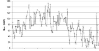
Figure 4: Q<sub>DAY</sub> measurements (◇) and computed values with day-average cycle (×)
