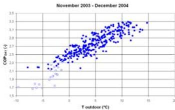
Figure 3: daily COP values (●: one compressor; ○: two compressors)
